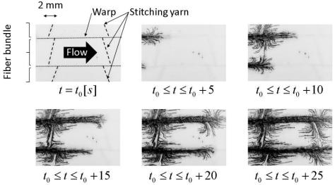
**Figure 1:** Progress of trajectories of particles suspended in epoxy under pressure difference  $\Delta P = -90 \text{ kPa}.$
